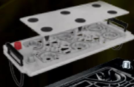
Integrated single point venting in the Labyrinth lid allows safe discharge of any gasses produced, while integral flame arrestors protect the battery from sparks and flames.
